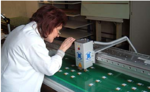
Figure 1: Soldering ribbon cables to the pad plane.
