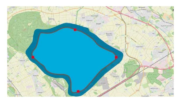
The future lake in the Hambacher Loch would have ebb and flow like the North Sea with a large underwater pumped storage power plant. A dam (black line) with sluices (red) could limit the tides in the shore zone to make it usable for recreational activities.
