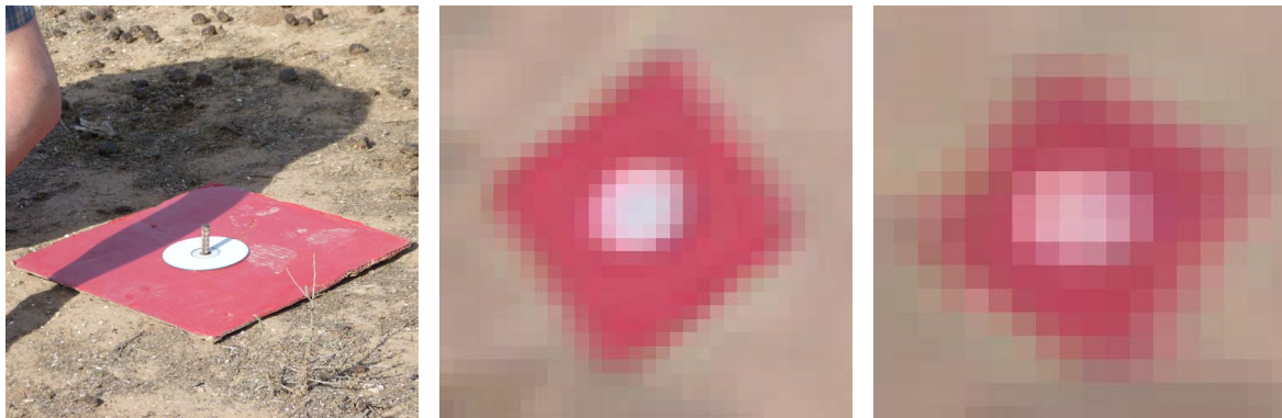
(a) Setup of a GCP using a metal pole, red cardboard and a CD (D'OLEIRE-OLTMANNNS ET AL. 2012: 3398) (b) GCP in aerial image from 105 m (c) GCP in aerial image from 190 m
