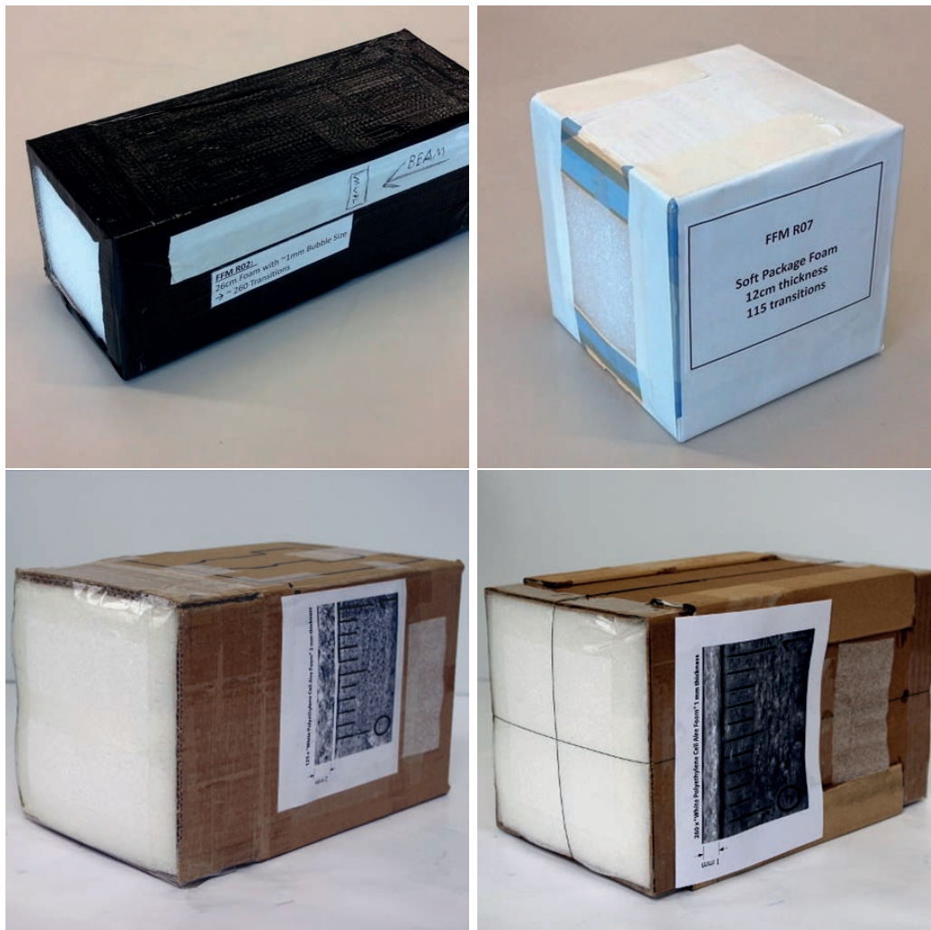
Figure 7.13: Photo of foam radiators type R002 (hard PE foam) top left and R007 (soft PE foam) top right. Type H lower left, Type N lower right.
